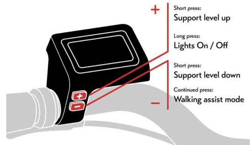
Finally, to turn on your front light, press and hold the + button for 2 seconds.
