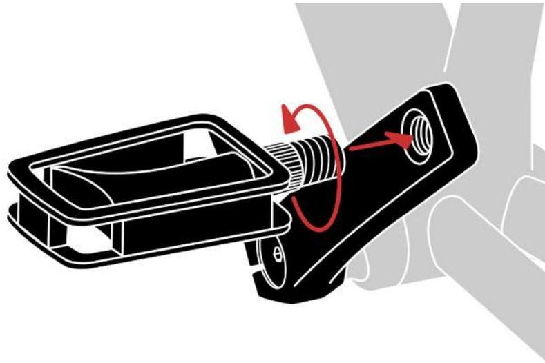
RIGHT pedal: this pedal has no indented lines and is smooth in between the pedal and thread.
