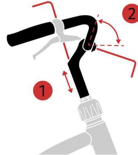
Tip: Should you wish to adjust the angles of your grips, brakes and shifter, you can do so with a simple turn of allen key 3 or 4. However, this should be correctly set already.
