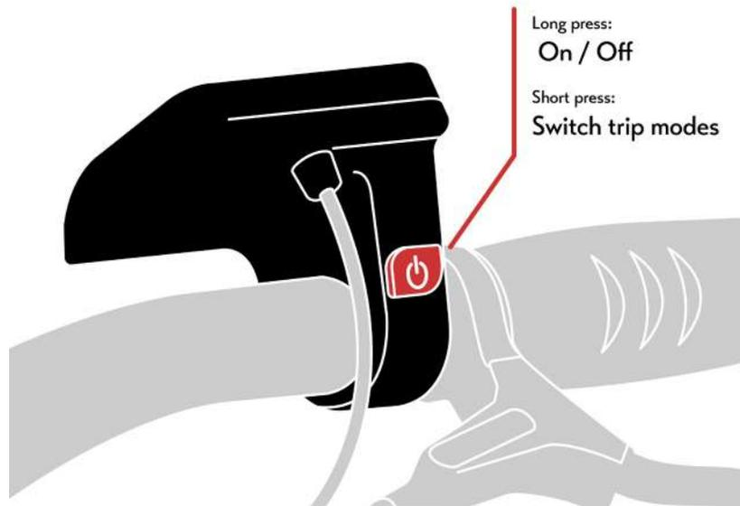
Once on, you can scroll through the 5 levels of motor assist using the + and - buttons on the front of the control module / display. For more in-depth instructions for your screen, please refer to the Bafang manual, found in PDF format on our website.
