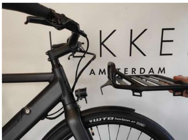
Please note: For the proper installation of the front rack, you need to remove the front light from its original holder and attach it to a longer version (see picture to the right). This holder is unfortunately only available from the 2nd week of August onwards. We will ship you the holder separately. Once you receive this holder, you can install the rack and lamp correctly. We recommend waiting with the installation of your front rack until you receive this holder!
