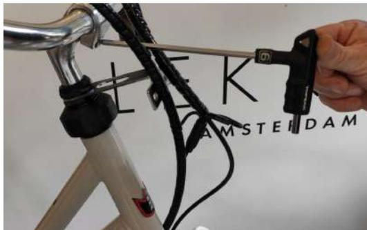
picture to the right. You might need to adjust the angle of the brakes and gear lever with a **3 and 4mm Alan key**.
